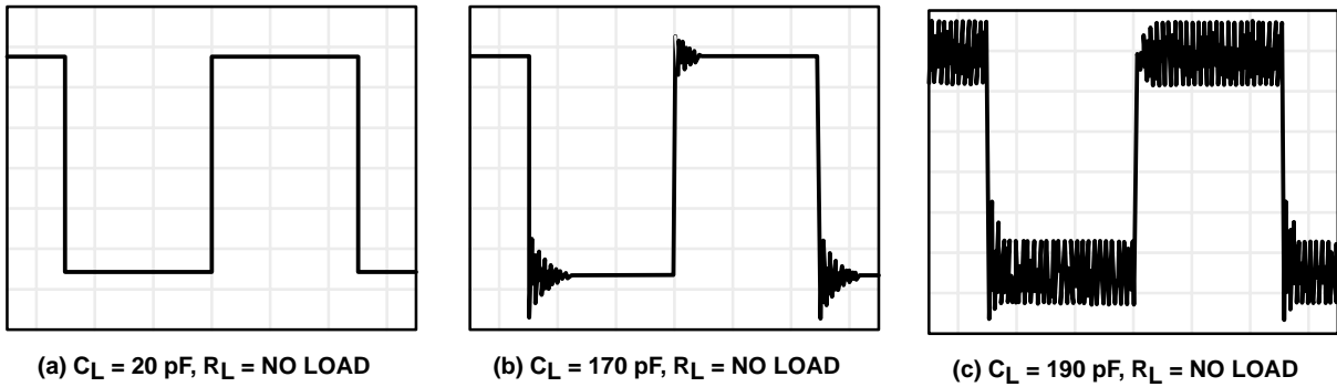
Figure 111. Effect of Capacitive Loads in Medium-Bias Mode
