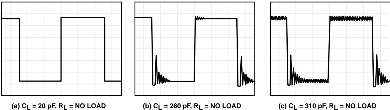
Figure 112. Effect of Capacitive Loads in Low-Bias Mode
